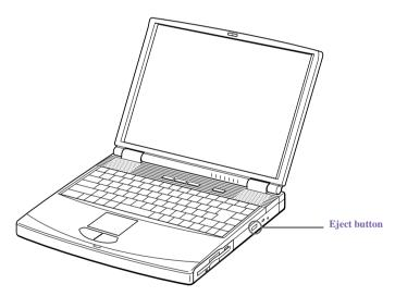
3 Place a CD or DVD on the tray with the label side facing up. For DVDs which can be played on both sides, the side of the disc facing up is the side that plays.
